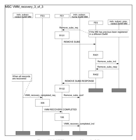
Figure 30.6: VMM recovery (sheet 3 of 3)
