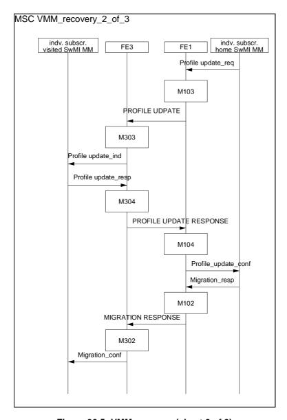
Figure 30.5: VMM recovery (sheet 2 of 3)
