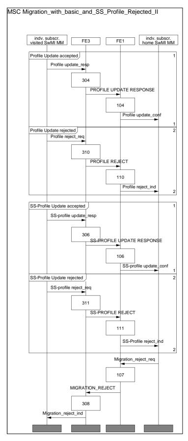
Figure 22.9: Migration rejection request upon receipt of the Profile update result and the SS-profile update result
