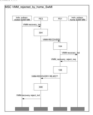
Figure 30.8: Rejection of VMM recovery
