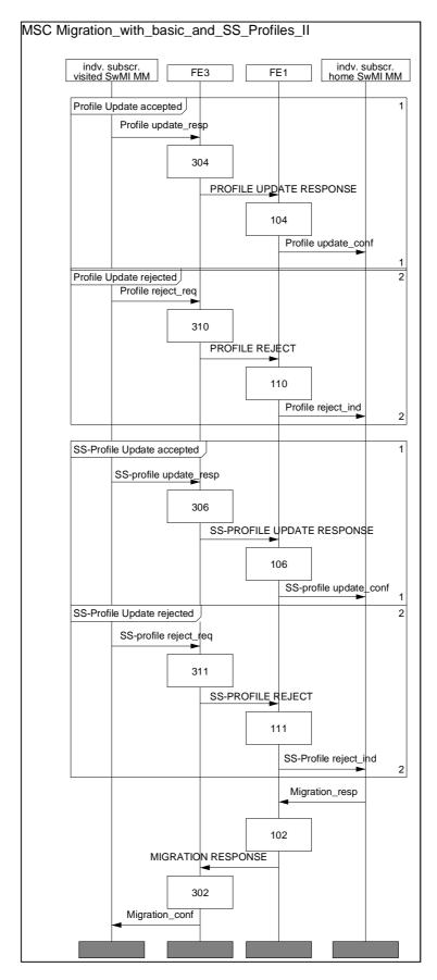
Figure 22.4: The SS-migration profiles exchanged before the final migration approval
