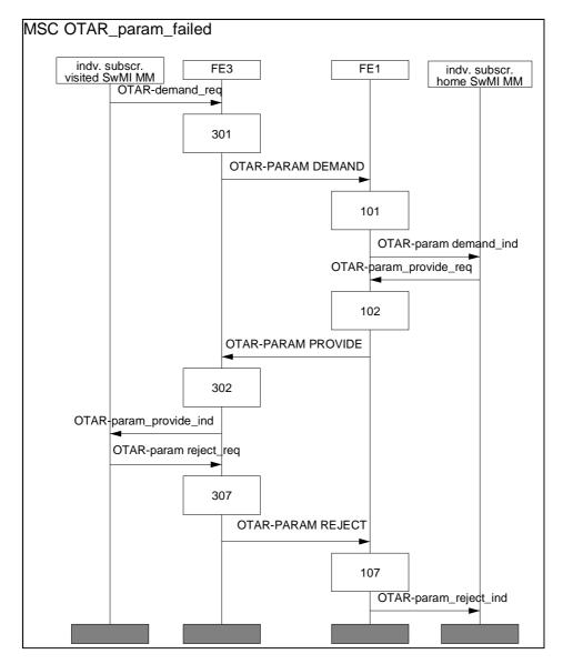
Figure 29.6: Failed OTAR SCK generation service
