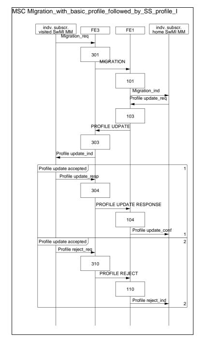
Figure 22.5: The SS migration profiles exchanged after the final migration approval
