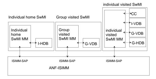
NOTE: The arrows illustrate the information exchange routes of the service. In the case of a solid arrow the information exchange is mandatory; in the case of a broken arrow the information exchange is conditional. The CC exists in the SwMI where the individual subscriber is now located (which might be the individual subscriber home SwMI or another individual subscriber visited SwMI) if the individual subscriber is engaged in a call when he migrates.
