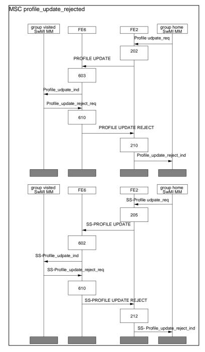
Figure 31.8: Rejection of profile updates in connection to group home SwMI MM initiated group attachment with migration profile exchange
