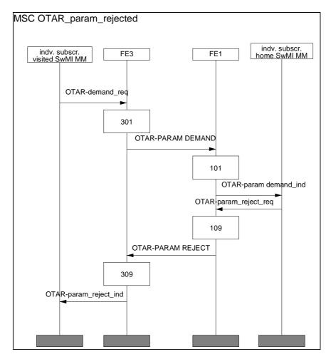
Figure 29.5: Failed OTAR parameter delivery
