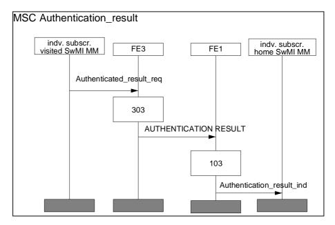
Figure 28.2: The successful subsequent authentication
