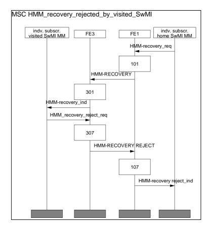
Figure 30.7: Rejection of HMM recovery
