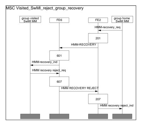
Figure 33.5: Rejection of G-HDR
