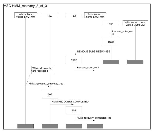
Figure 30.3: The HMM recovery (sheet 3 of 3)
