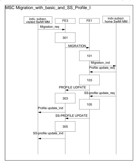
Figure 22.3: The SS-migration profiles exchanged before the final migration approval
